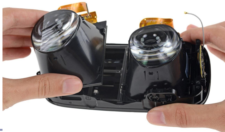
Teardown of an Oculus Rift CV1 showing details of lenses and displays https://www.ifixit.com/Teardown/Oculus+Rift+CV1+Teardown/60612
